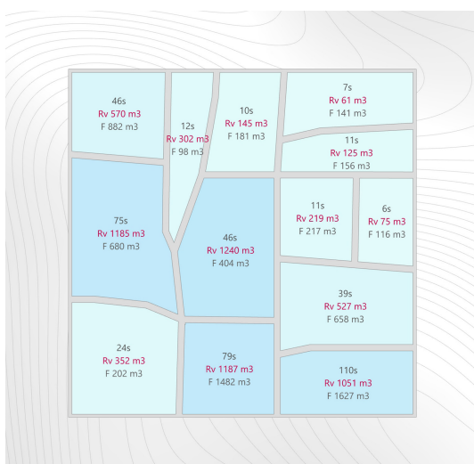
Fig. 3.12b Runoff Volume & Cumulative Infiltration Map
