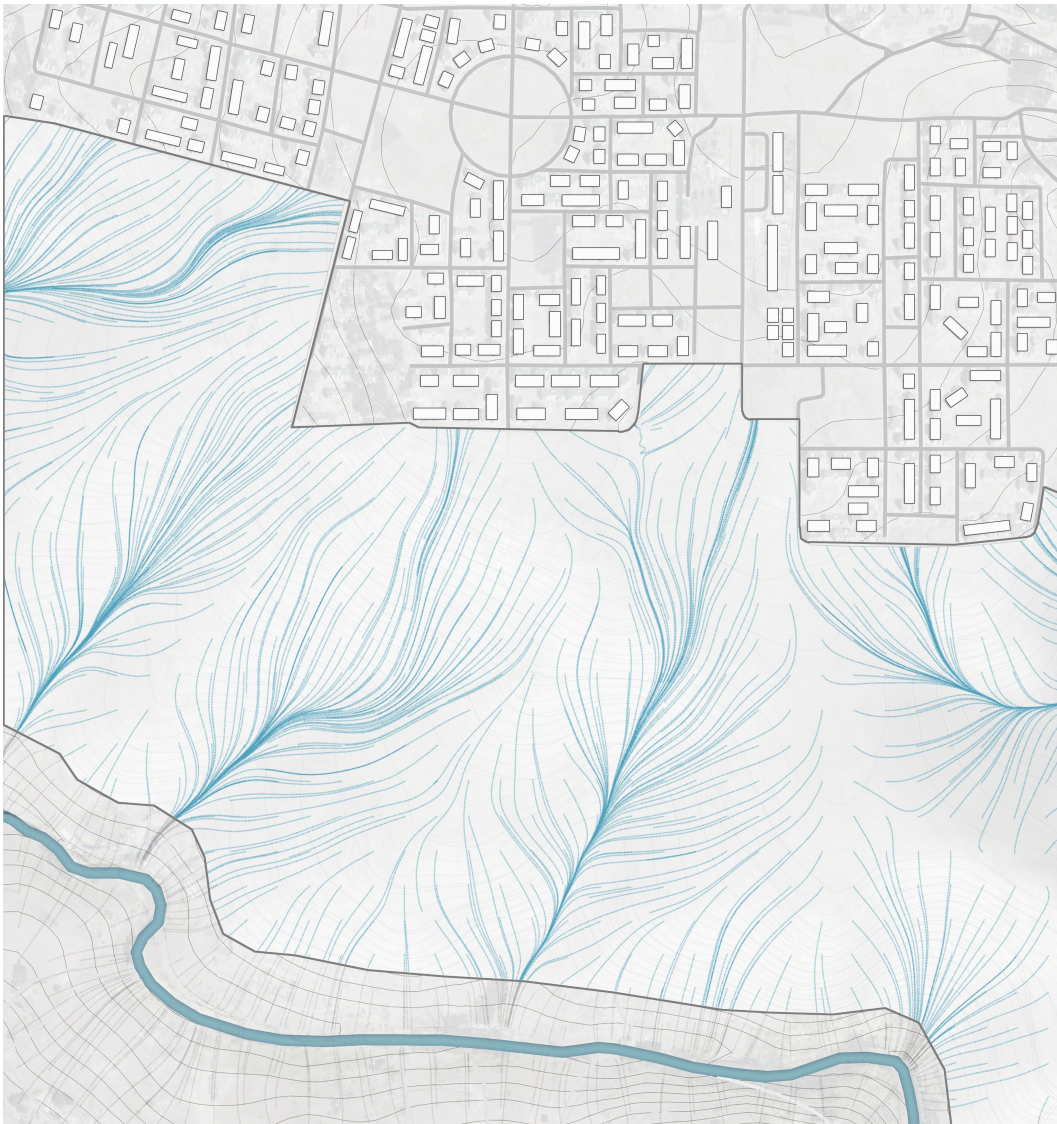
Fig. 4.3 Numerical Based Rainwater Flow Direction Network
