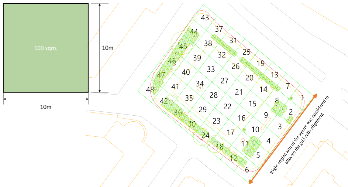
Figure 17: Assigning the standard cell into one of the selected public places before survey.
