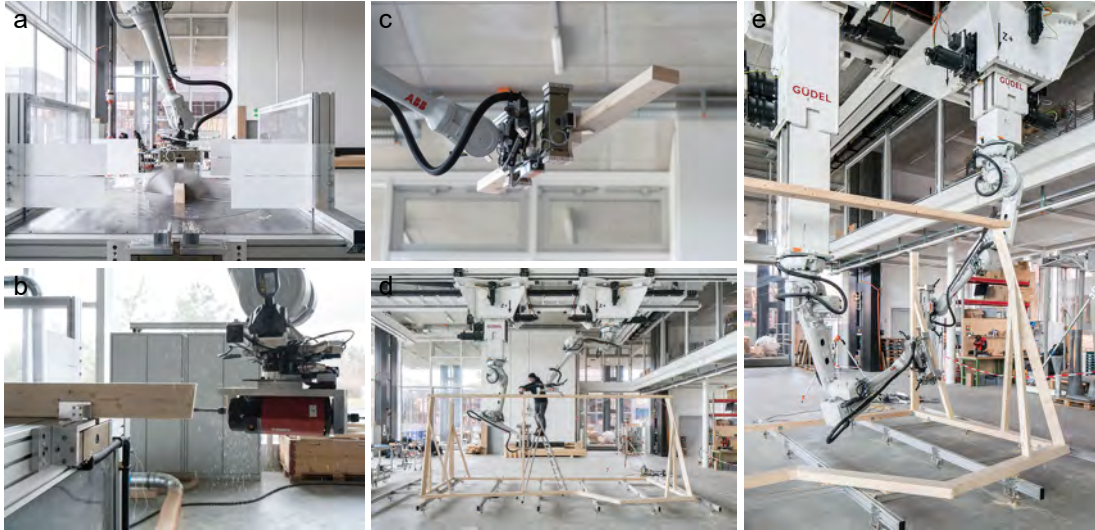
Figure 2.5: Collaborative Fabrication of a timber frame module. a) CNC-saw cutting a beam in cooperation with a robotic arm, b) Pre-drilling a screw hole, c) Robotic arm carrying a beam to its final position, d) Robotic assembly of the bridge technique, e) Cooperative robotic assembly of the corner technique. Photographs by NCCR Digital Fabrication / Roman Keller, 2018.
