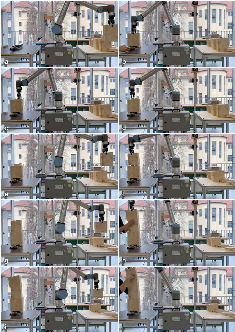
Figure 4.25: Collaborative assembly procedure: a) & b) Pick and place of the first offcut, c) & d) Placing the tenon joints, e) & f) Pick and place of the second offcut, g)–j) Pick and place of the third and fourth offcuts with human collaborator inserting the spline joints.
