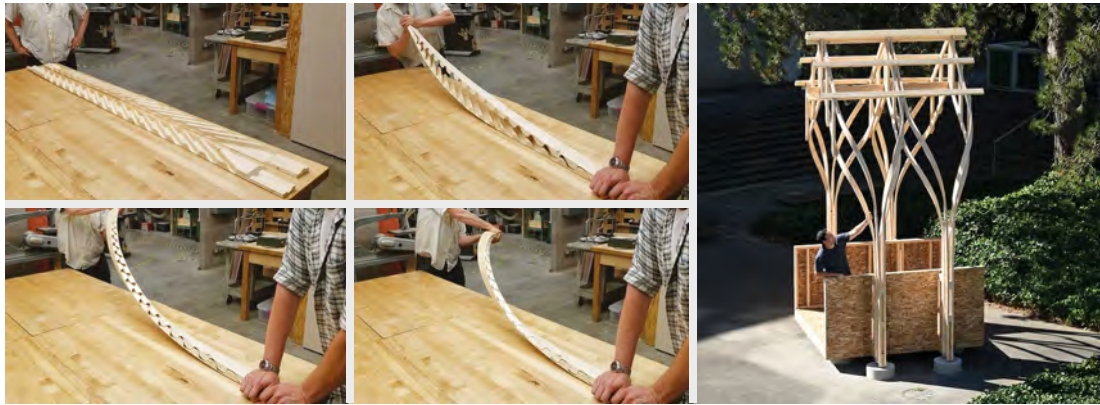
Figure 2.11: Left: Team members demonstrate the bending of a two-by-four prepared for use in the pavilion prototype. No steaming or soaking was required to bend the member. Members are glued and vacuum-bagged. Right: One Bay Prototype. Photographs by Blair Satterfield et al., 2020.
