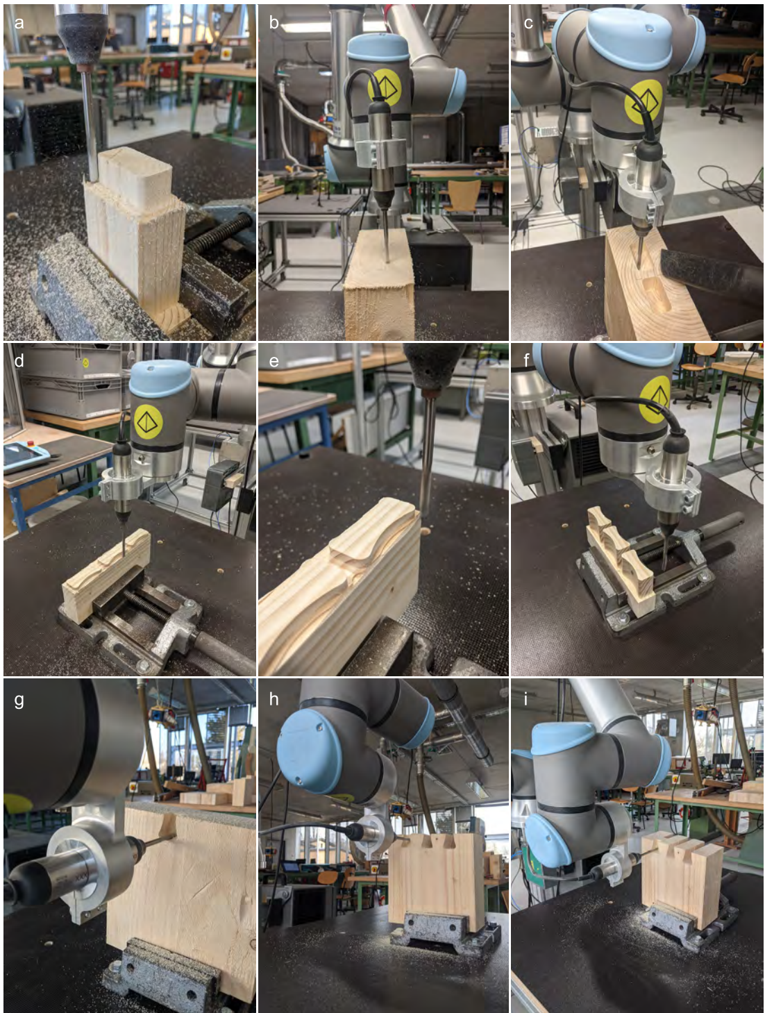
Figure 4.23: Robotic fabrication procedure: a) Tenon joint, b) Angular surface, c) Tenon joint pocket, d)–f) Spline joints, g)–i) Spline joint pockets.
