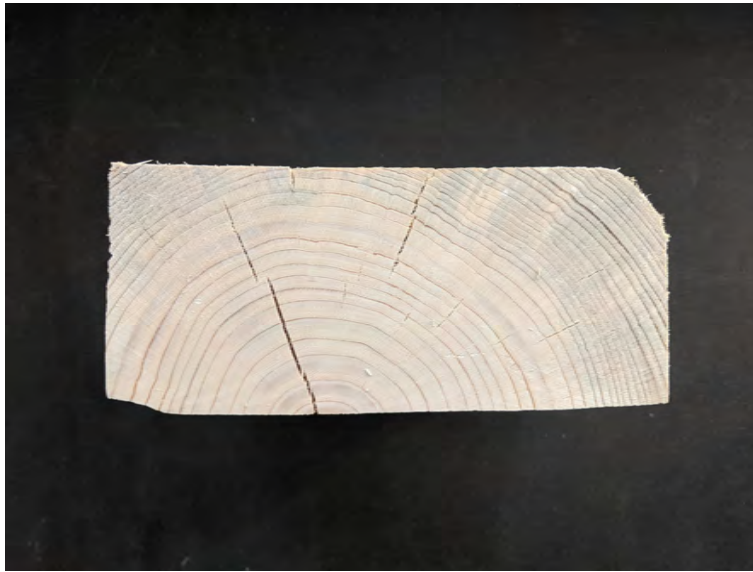
Figure 1.4: Offcut with cracks and blue mold.
