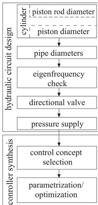
Figure 3: Process of hydraulic control systems design.
