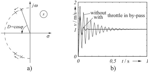
Figure 5: Eigenvalues (a) and step response (b).
