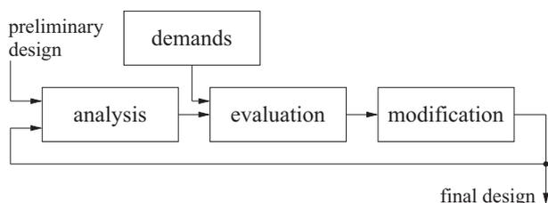
**Figure 1:** Iterative process of control system design.
