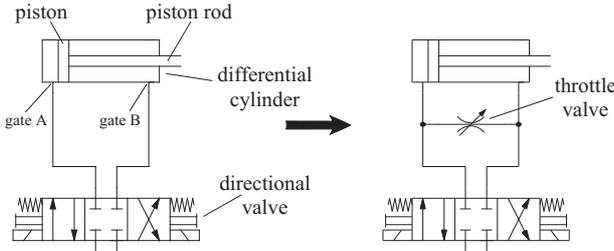
Figure 4: Circuit set-up before and after modification.
