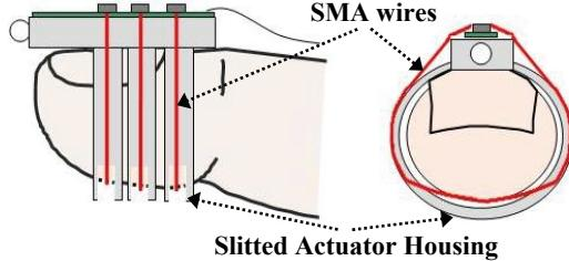
**Figure 2: Schematic view of a thimble device**
