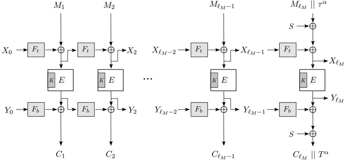
**Figure 6.1.:** Schematic illustration of the encryption process with POET for an  $(\ell_M)$ -block message  $M = M_1, \dots, M_{\ell_M}$ , where  $S$  denotes the encrypted message length, i.e.,  $S = E_K(|M|)$ ,  $F$  is an  $\epsilon$ -AXU family of hash functions, and  $\tau^\alpha$  is taken from the most significant bits of the header processing to pad the final message block. Note that the functions  $F_t$  and  $F_b$  use the keys  $L_F^{top}$  and  $L_F^{bot}$ , respectively.
