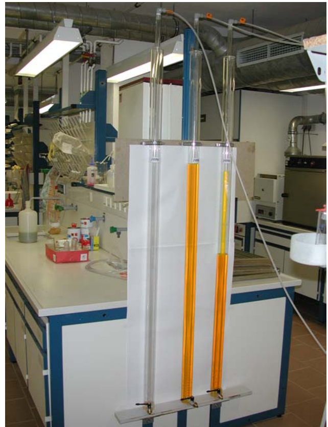
Figure 3 Air trapping (left: empty, middle: filled, right: vacuum)
