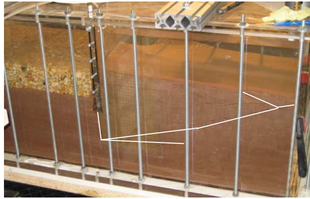
Figure 8. Result after failure (white line = slip plane)
